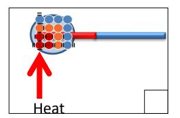
Conduction happens quickly in metals, for example in frying pans when cooking.
