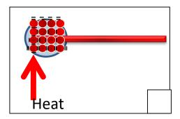
Conduction cannot happen in gases because the particles are too far apart. They are insulator 5
